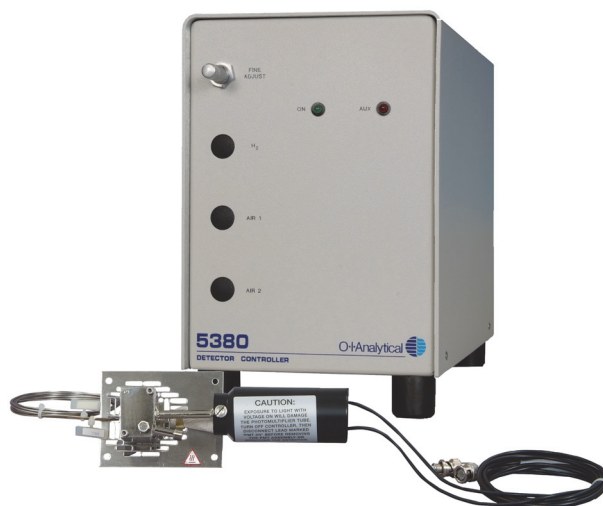
Figure 1. OI Analytical 5380 Pulsed Flame Photometric Detector
